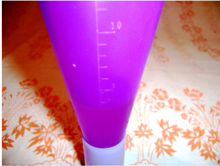
Figure 7: The calibrations on rain gauges are not very fine or accurate
