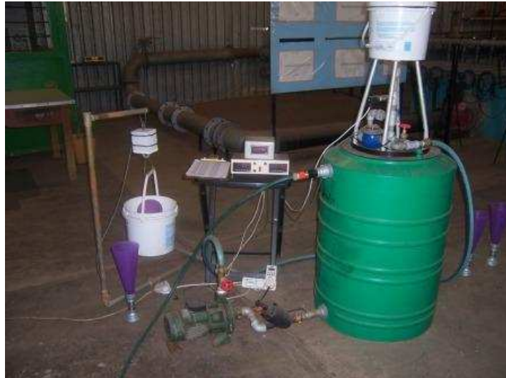
Figure 6: Components of the mobile sprinkler test bench
