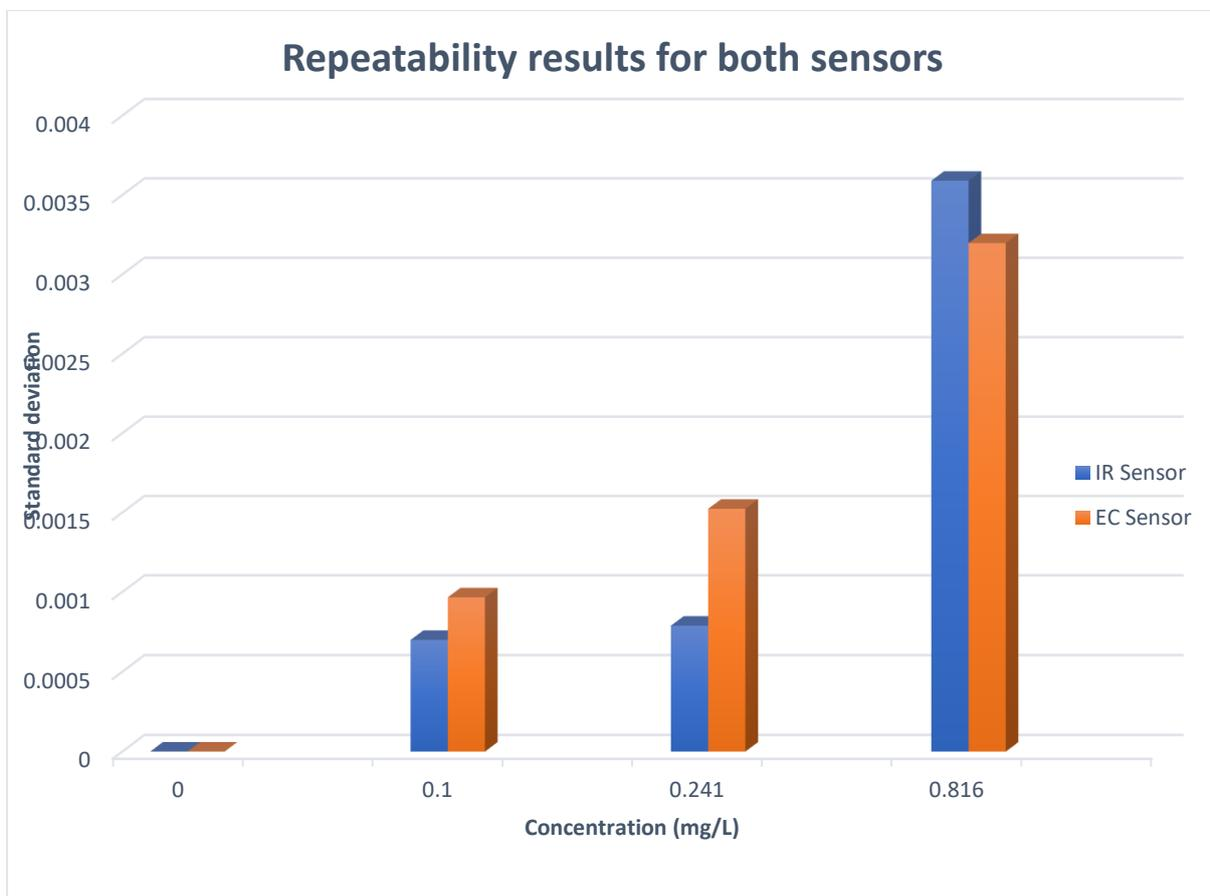
Figure 1. Repeatability data for both sensors.
