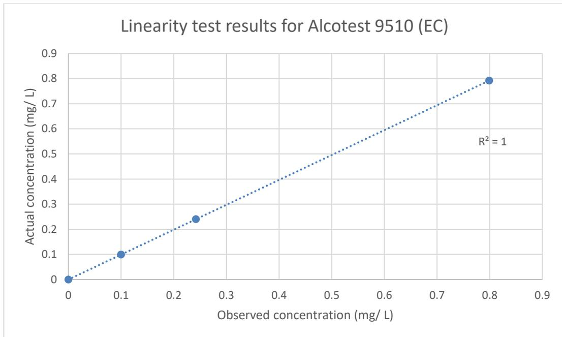
Figure 5. Linearity test for Alcotest 9510 (EC)
